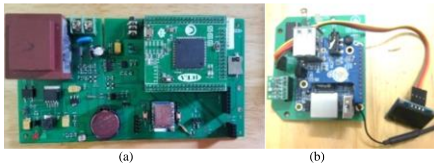
Figure 9. Designing of the (a) LMD board and (b) AMD board
